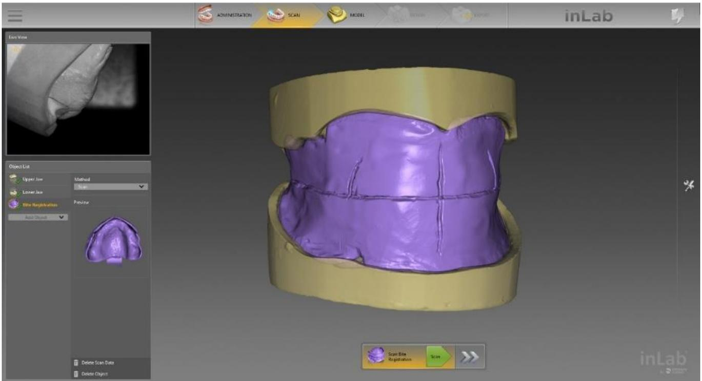
A new holder developed especially for digital dentures positions the bite registration in the inEos X5 scanner for reliable, shake-free scanning in just one step. A new scan algorithm allows all the relevant information to be captured precisely. The new scan object "Bite registration" precisely aligns the upper and lower jaws.
