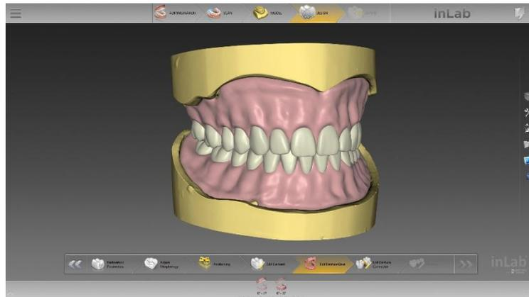
This technique has been used to design fixed restorations with great success for years. Specifically, it involves an algorithm that the software uses to propose an accurate restoration design to the dental technician based on the existing jaw situation. This central element of the inLab software is now also being used for full dentures.
