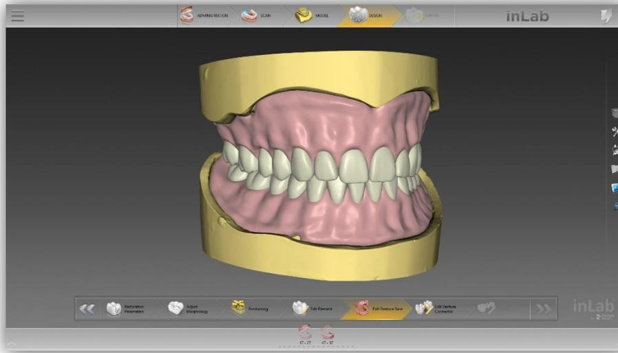
The inLab SW 20.0 offers two options for tooth placement: the use of digitized denture teeth that are stored in a tooth library, or individual tooth set-up. Both are based on the unique biogeneric algorithm through which the software already adapts the preoccluded denture teeth to the given jaw situation.
