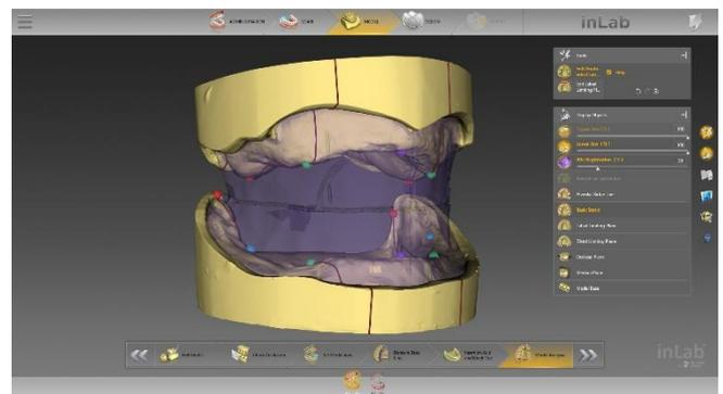
In the "Model analysis" step, the software displays anatomical landmarks automatically based on the digitalized jaw situation. The anatomical landmarks, such as the position of premolars, papilla incisiva, tubers and retromolar pad can be corrected manually. The initial proposal of the tooth set-up is based on alignment of the models and the model analysis. If the help option is activated in the inLab software, additional graphics and help texts for the model analysis will be displayed.
