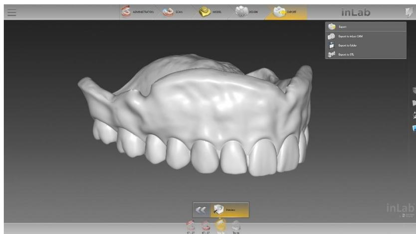
In the export phase, the denture base and tooth arch for the upper and lower jaws as well as the optional try-in is displayed in the Restoration Selector at the bottom. As usual, these can be transferred seamlessly to inLab CAM 20 or exported as STL data via side menu.
