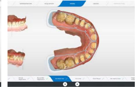
Setting the model axis and insertion axis are key for best grinding of restorations in the manufacturing phase.
